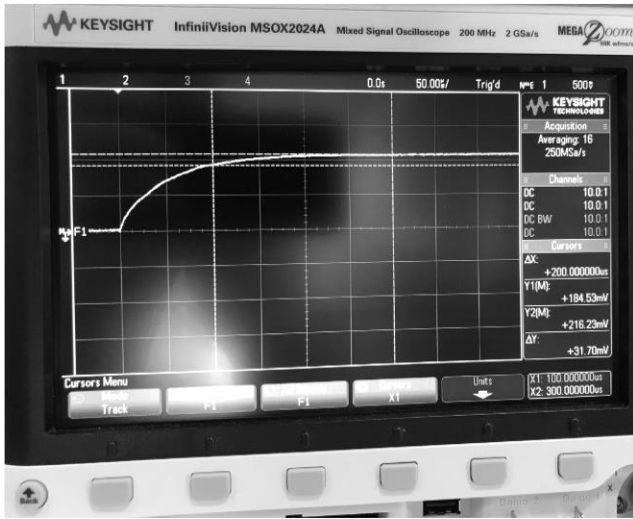
Fig. 4 Coil current transient in optimal power consumption mode. R_s=1 Ohm
